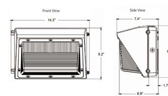
The QLS Wall Pack is a rough and ready tool to ensure your building is well lit, and your people are safe. Offering a tough, weatherproof, aluminum frame with a clear polystyrene lens, this wall pack offers superior light protection, while its 144 LEDs reduce cost and greatly improve product life. Fits to existing wall pack hardware for quick remounts. Available with a state of the art microwave photocell that switches light output based on occupancy between 10% to 100%.
